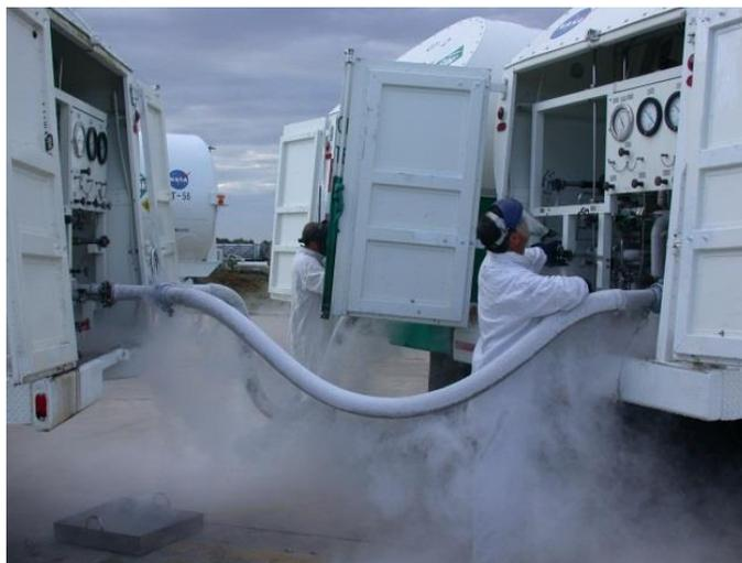
**Figure 13: The production of liquid breathing air from liquid oxygen and liquid nitrogen tankers (Doerr et al, 2013)**
