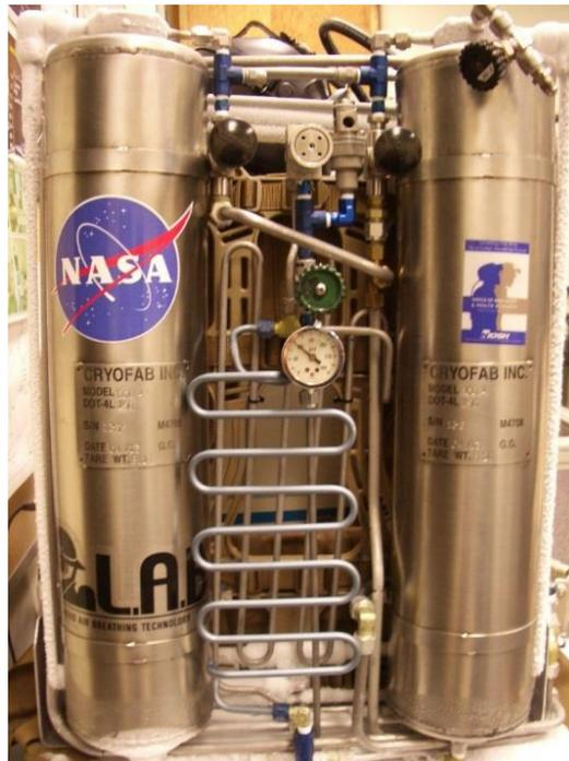
The CryoBA program is an advancement of the current liquid air SCBA design that
