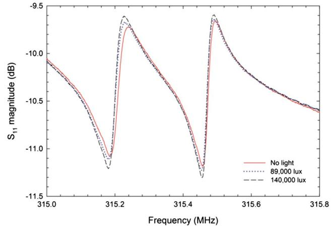
FIG. 9. (Color online) Different values of illuminance are measured using a single sensor tag loaded with a photodiode. Changing light intensity is indicated as a shift in the  $S_{11}$  magnitude and demonstrates sensor operation while affixed to the surface of a cylinder.
