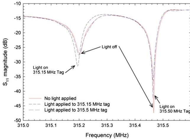
FIG. 10. (Color online) Incident  $S_{11}$  measurements at the network analyzer demonstrate that a pair of tags separated in operating frequency by 350 kHz is capable of individually sensing light vs dark conditions.
