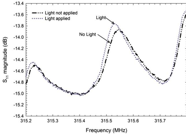
FIG. 7. (Color online) Measured  $S_{11}$  signals indicate an increased magnitude at the 315.50 MHz peak, representing illuminated conditions and decreased magnitude corresponding to decreased illumination.
