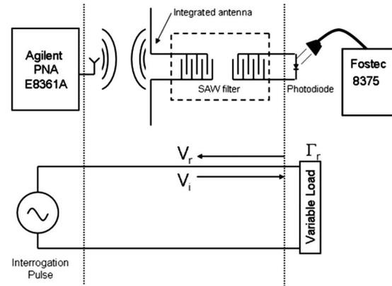
FIG. 6. (a) Network analyzer is used as an interrogation unit to both generate the ping signal and receive the reflected  $S_{11}$  signal. The wireless link can be modeled as a transmission line with a variable impedance load, which causes a varying reflection coefficient ( $\Gamma_r$ ). (b) Analysis of the reflected signal allows the sensor state to be determined.
