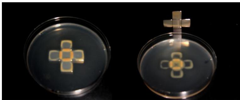
Fig.2 Photograph showing the assembly of complex shapes of Fe doped in HA using the citrate capping synthesis technique.
