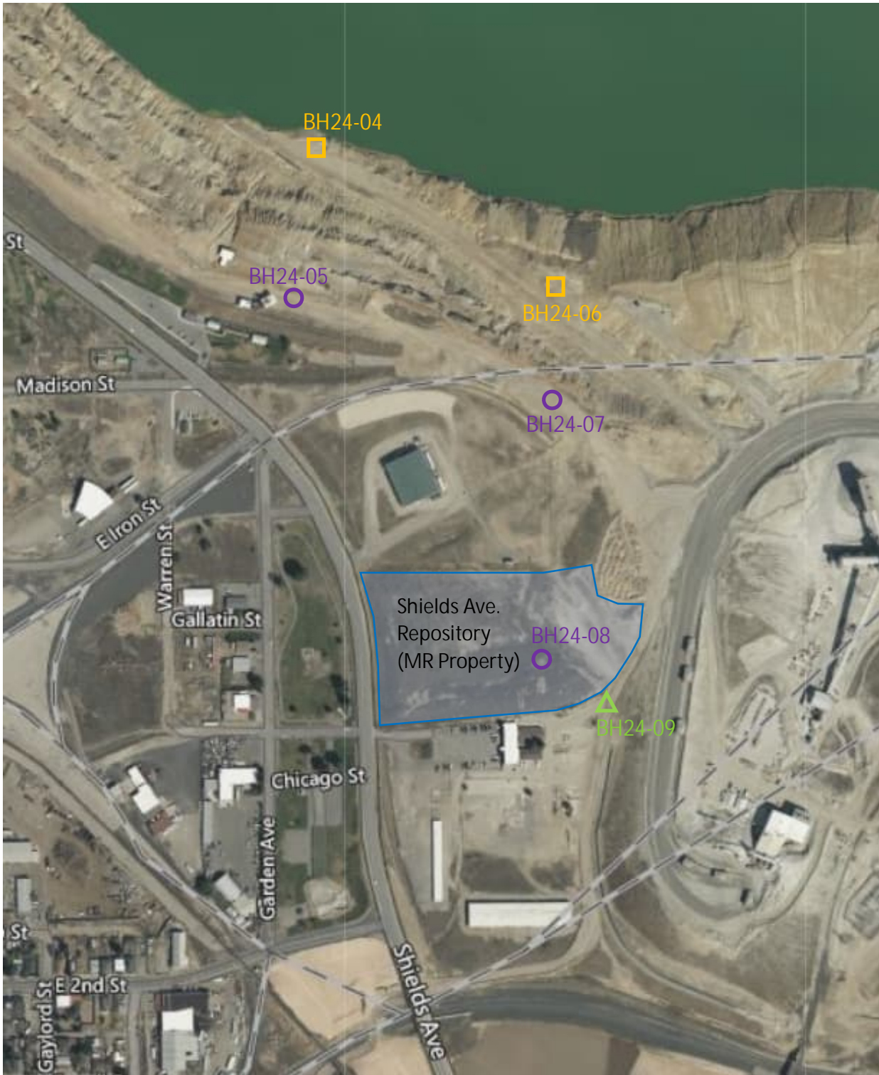
Figure 2. Shields Avenue Repository (circle), South Ramp (square), and Slurry System Piping (triangle) Proposed Borehole Locations.
