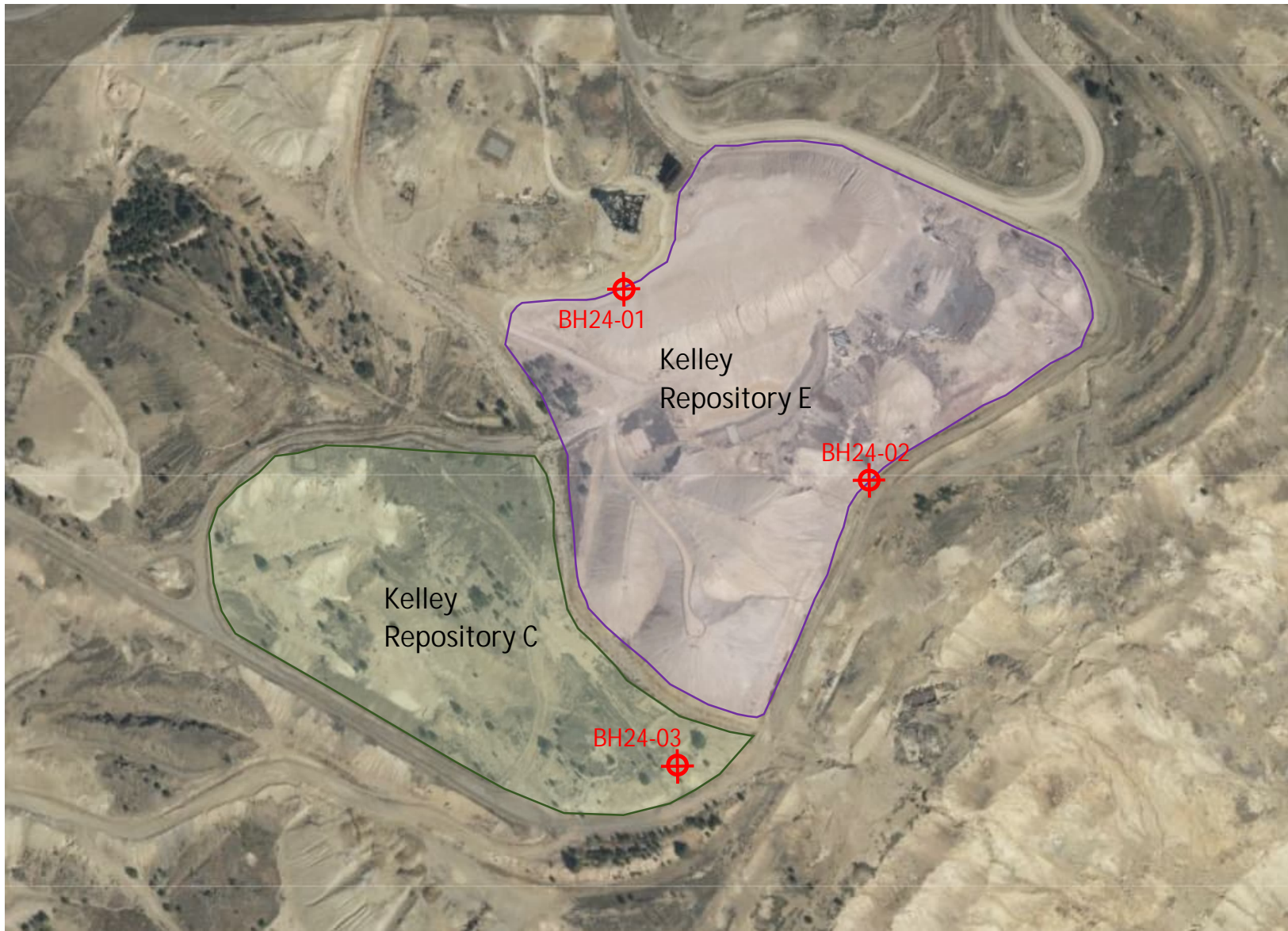
Figure 1. Kelley Mine Area Repositories C and E Proposed Borehole Locations.
