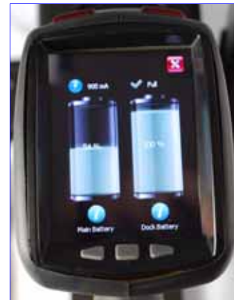
Battery Status Screen (Delta inserted in DDS)
