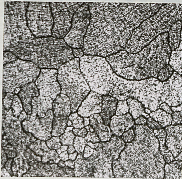
Fig. 12 - Specimen 2 A. As cast. Magnetic. X231
