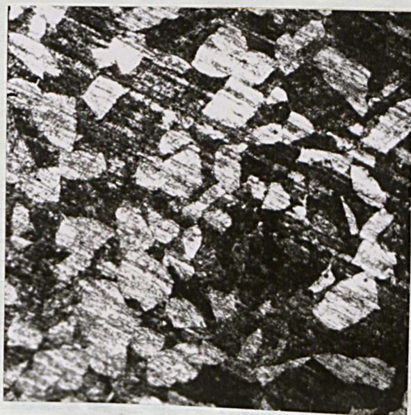
Fig. 20 - Specimen 3 G. Annealed at 750^{\circ}\text{C} for 4 hours and quenched at 20^{\circ}\text{C} . Not magnetic. X231.
