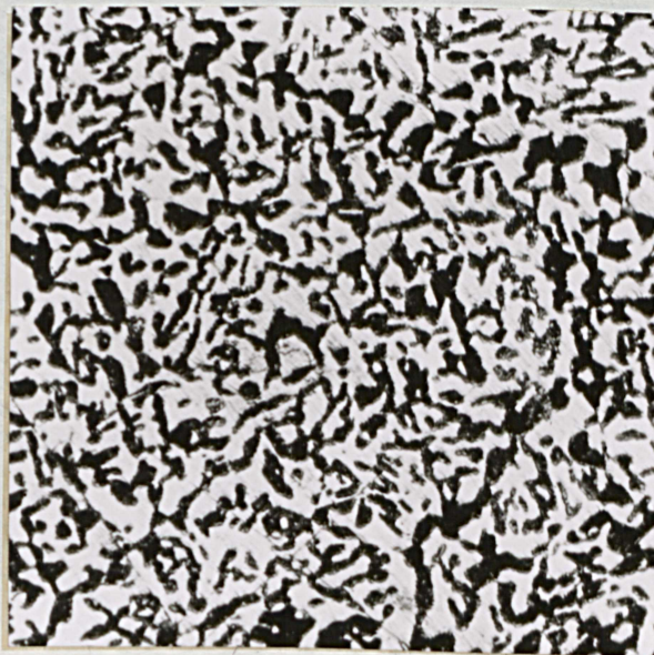
Fig. 10 - Specimen 1 I. Annealed for 4 hours at 650°C and quenched at 20°C. Not magnetic. X231
