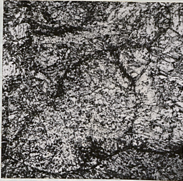
Fig. 18 - Specimen 3 A. As cast. Magnetic. X231.
