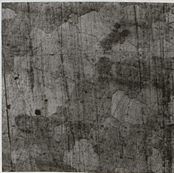
Fig. 17 - Specimen 2 J. Annealed for 4 hours at 600°C and quenched at 20°C. Not magnetic. X231.
