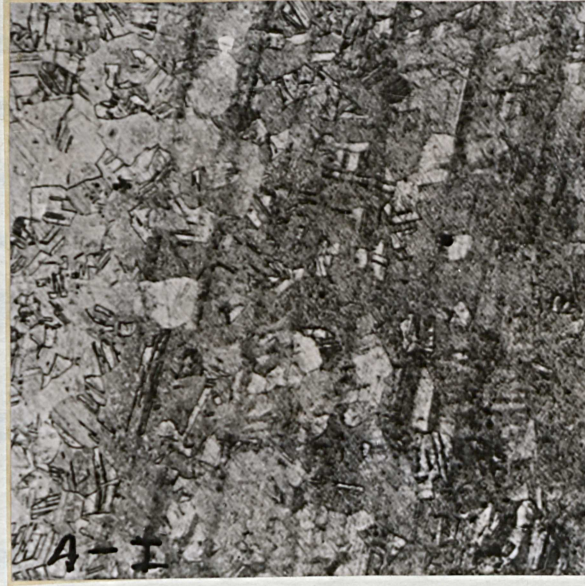
Fig. 28 - Specimen 4 I. Annealed for 4 hours at 650°C and quenched at 20°C. Not magnetic. X231.
