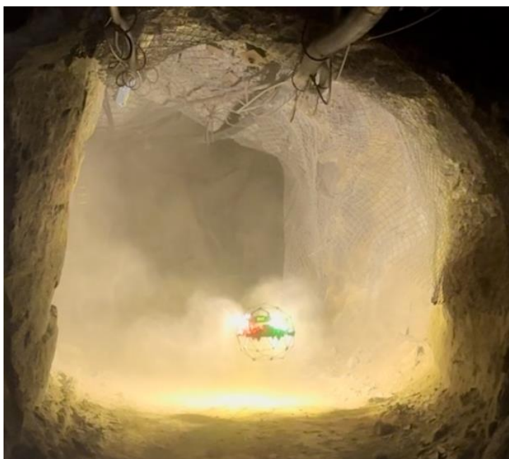
Figure 26: Elios 2 Dust Cloud
