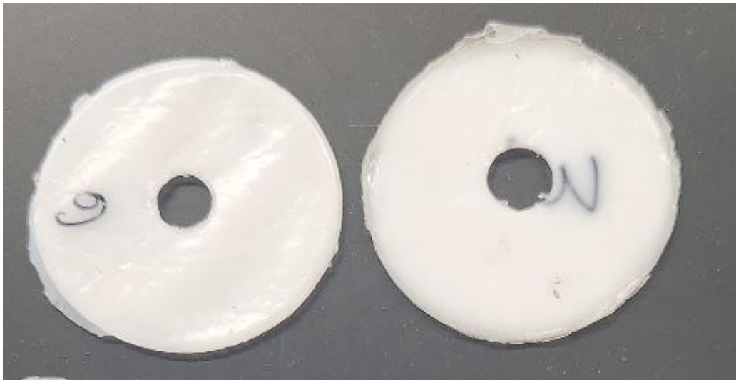
Figure 15: PCL Shear test sample prior to testing.
