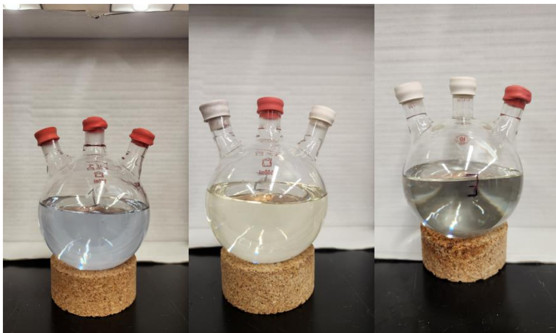
Figure 7: Individual polymerization attempts utilizing excess catalyst and radical initiator in attempt to propagate and excite reaction for polymerization reaction. Color difference indicate changes in exceeding amounts of catalyst and radical initiator.
