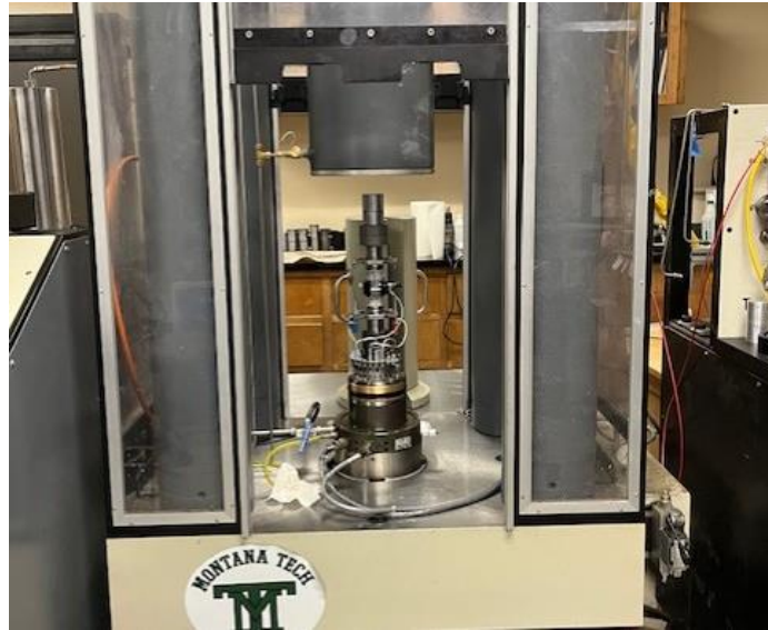
Figure 12: The load frame with the specimen in a wrapped membrane so no oil can penetrate the specimen
