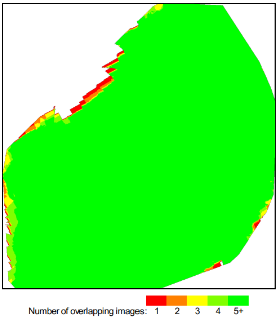
Figure 4: Number of overlapping images computed for each pixel of the orthomosaic. Red and yellow areas indicate low overlap for which poor results may be generated. Green areas indicate an overlap of over 5 images for every pixel. Good quality results will be generated as long as the number of keypoint matches is also sufficient for these areas (see Figure 5 for keypoint matches).
