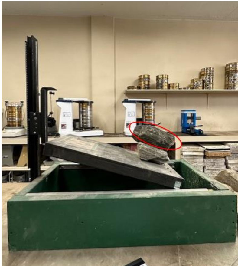
Figure 15: Tilt test machine with two hand samples from the Madison Dam rock mass
