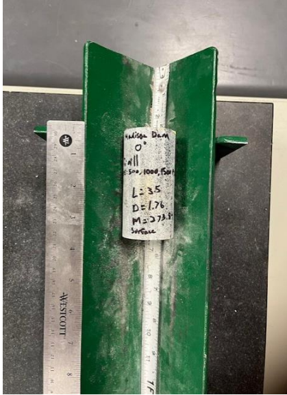
Figure 11: Specimen used for the multistage triaxial test cored parallel with the bedding planes.
