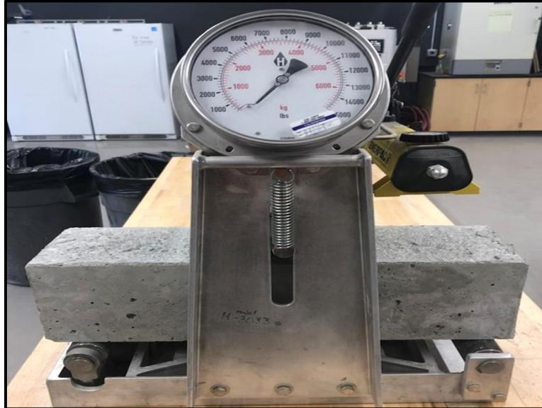
*Figure 21 - 4-Pt Bending Strength Tests*
