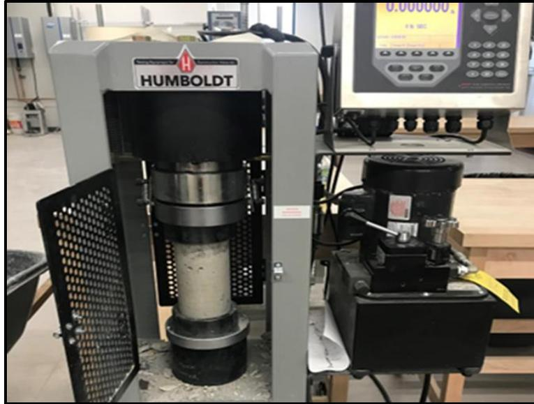
*Figure 20 - Compressive Strength Test Frame*
