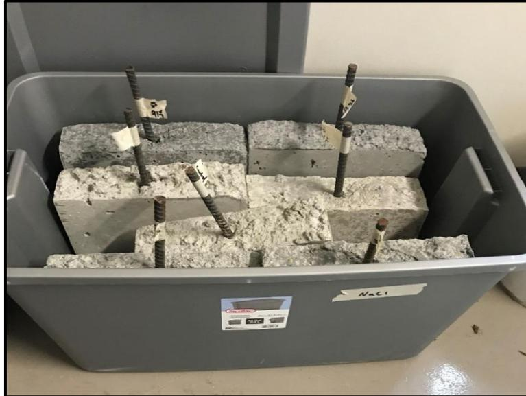
*Figure 14 - Samples in Solution for Wet OCP Measurements*
