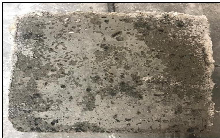
*Figure 22 - Example of Typical Salt Scaling on  $\text{Na}_2\text{SO}_4$  Samples*
