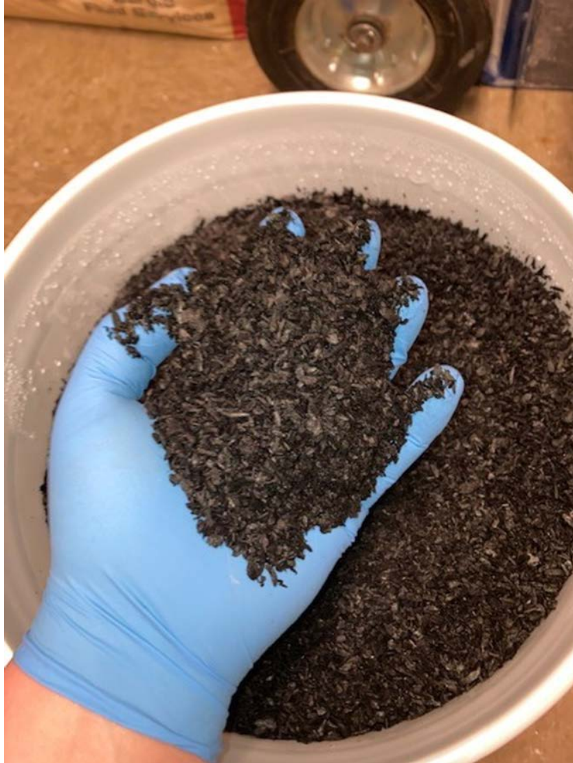
Figure 9: Picture of Biochar Material Used During Experimentation
