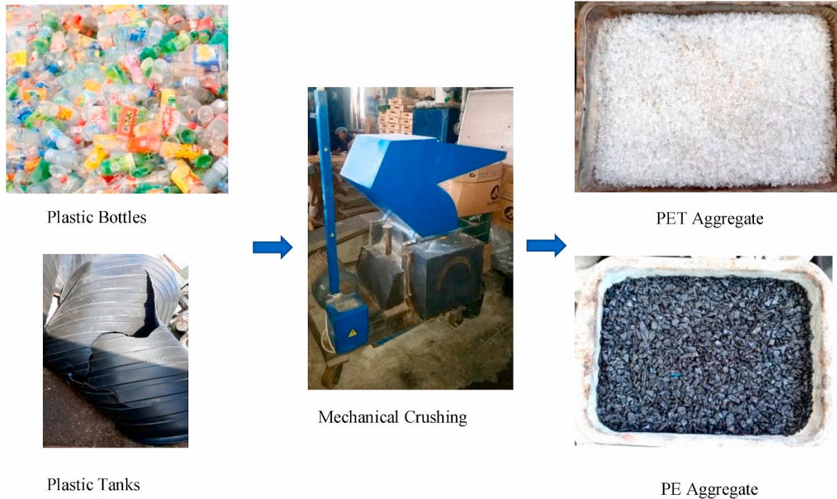
Figure 4: Recycling process of PE and PET wastes (Tayeh et al., 2021)
