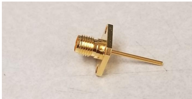
Figure 11: Straight-jack connectors used to launch the waveforms into the waveguides
