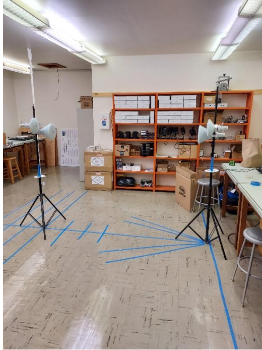
Figure 25: Indoor path-delay experimental setup, used to test differences between both sets of antennas
