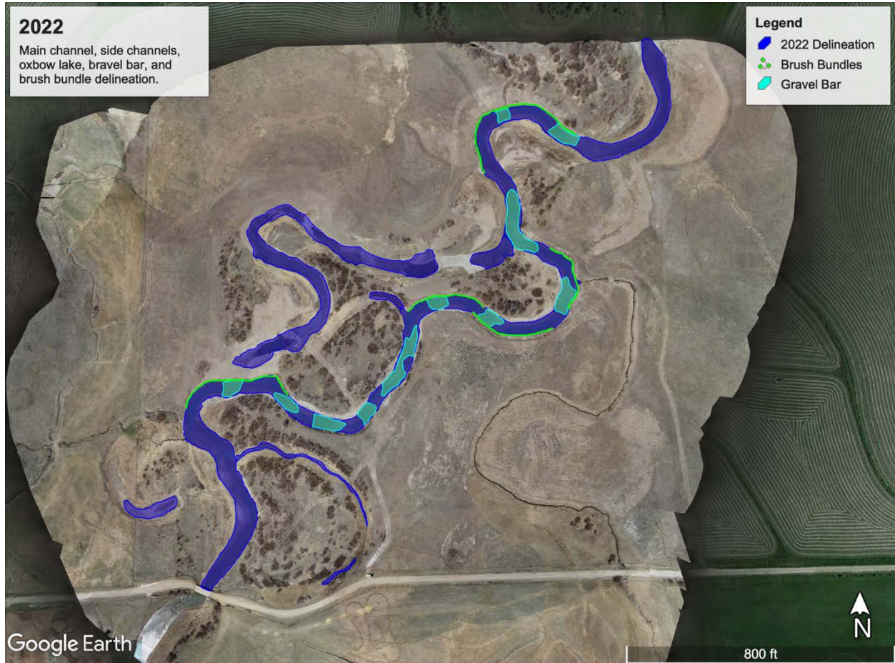
Figure 23: Restoration techniques brush bundles and plug and pond using gravel bars delineated from 2022 drone data overlaid on 2014 satellite data
