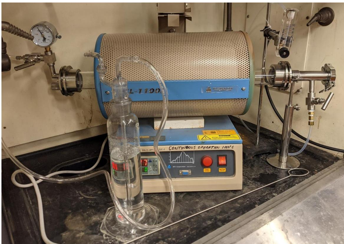
**Figure 58: Tube furnace setup used for calcination in oxygen environment. After flowing through the furnace, gases are flowed through a bubbler tube to prevent backflow into the tube and maintain pure oxygen atmosphere. For reactions in air, the bubbler is removed and the flange vents are opened to the ambient atmosphere.**
