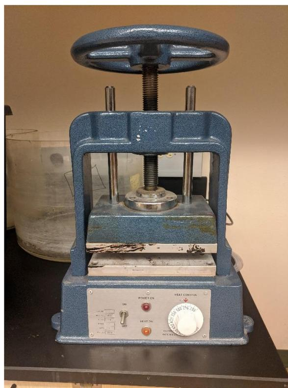
**Figure 57: Manual hot press used for post-processing of electrospun fibers. To tighten uniformly, the press is turned 1/4 rotation after first contact with the sample.**
