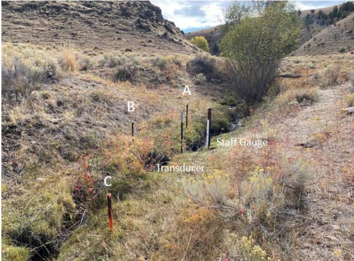
Figure 6: Groundwater monitoring site setup at Site 3. Wells at each site are labeled alphabetically from up to downstream.
