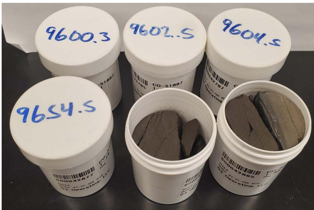
Figure 16: Bakken core sample jars with labeled depths.
