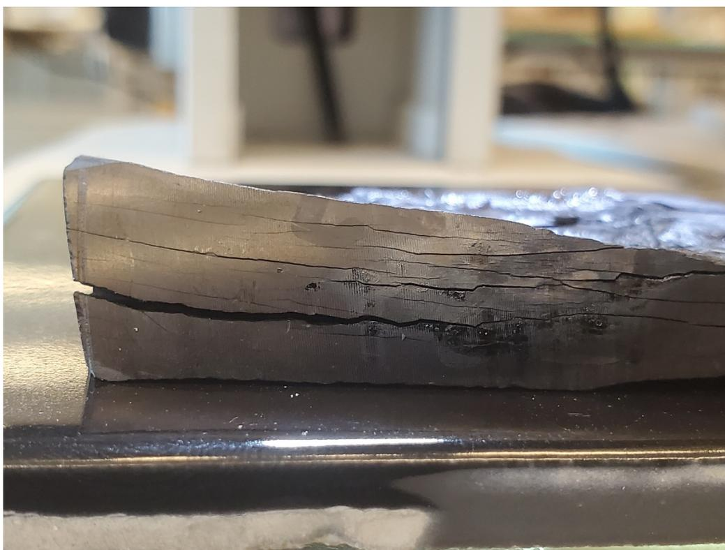
**Figure 27: Bakken core 9600.3 #1 fracture growth.**
