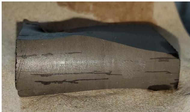
**Figure 32: Bakken core 9654.5 #1 water absorbed via fractures.**
