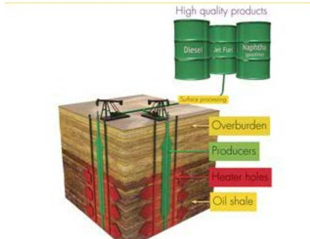
Figure 13: Shell's In-situ Conversion Process project visual representation (INTEK, 2011).
