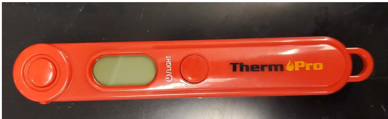
**Figure 21: Probe thermometer, used to measure liquid temperatures.**
