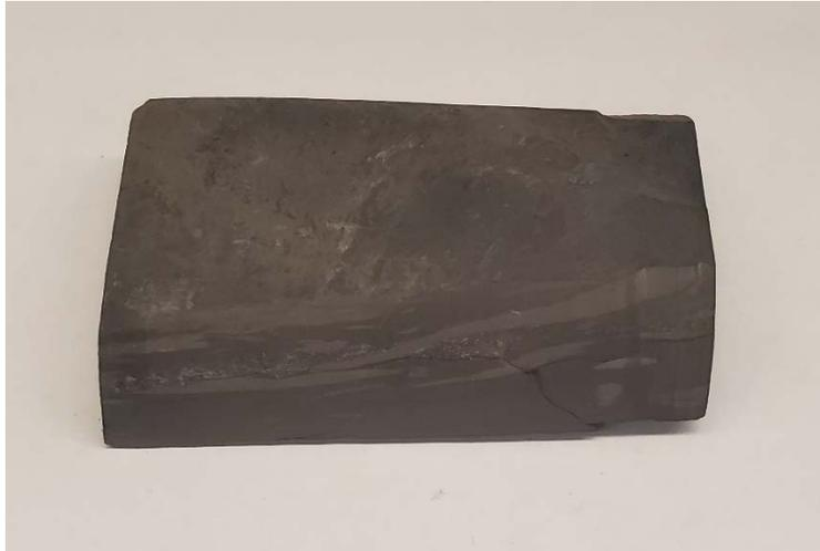
**Figure 25: Bakken core 9600.3 #1 prior to EMR exposure.**
