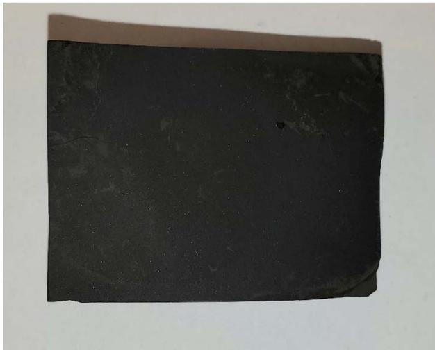
**Figure 33: Bakken core 9654.5 #2 prior to 100% power water bath test series.**
