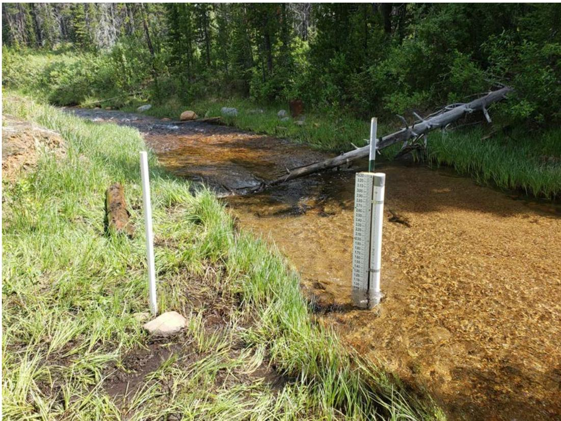
**Figure 10: Photo of staff gage/stilling well and piezometer placement at EC3**
