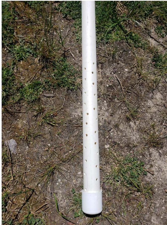
**Figure 12: Picture of capped piezometer base**
