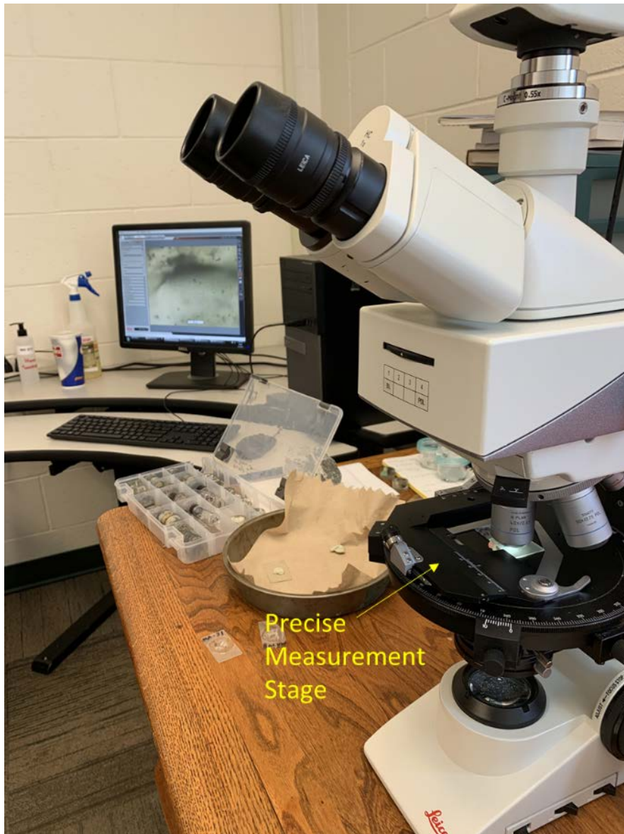
Figure 14. Precise measurement stage on a petrographic microscope.
