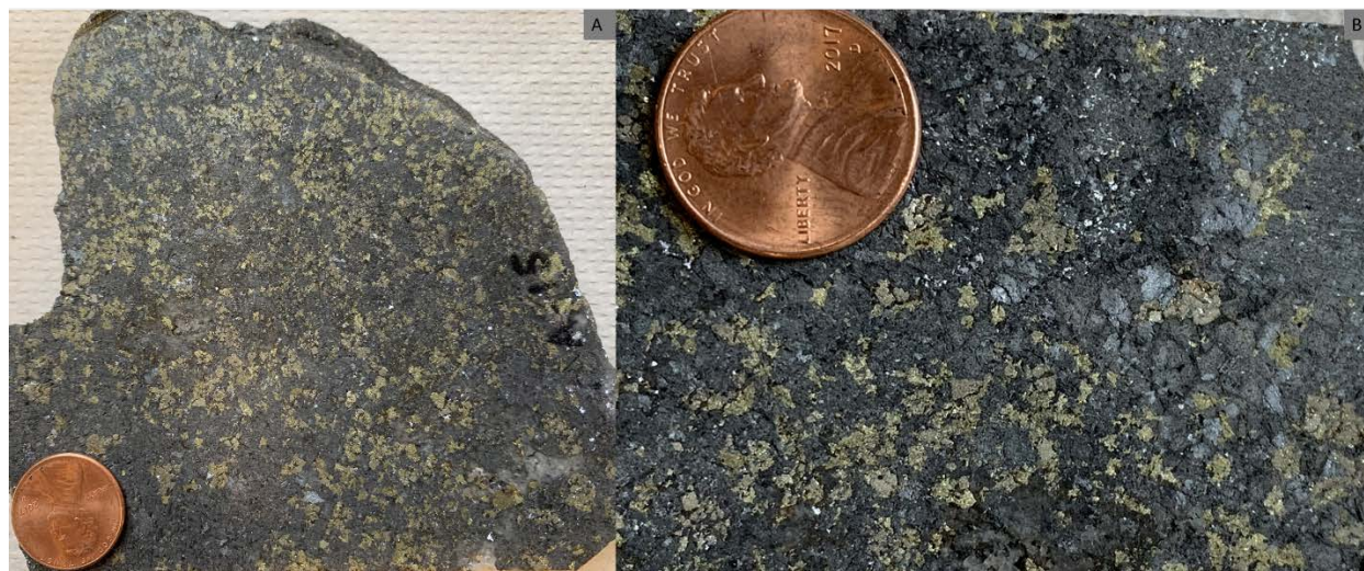
Figure 32: A) Massive sulfides from Marget Ann sample MA-15. B) Closer image of sample in photo A, dark gray is a mix of sphalerite and galena, and the yellow/gold is pyrite and chalcopyrite.
