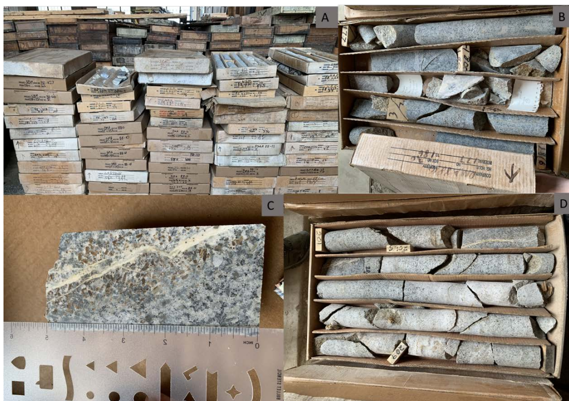
Figure 11. A) Core boxes from the Blackjack Silver collection located in the Badger Hoist building. The samples were originally collected by the New Butte mining company. B) Core box DMA 88-10, box 20, depth interval between 177 ft. and 186 ft. C) Example of core sample used to make plugs for micrographs and SEM-EDS. D) Mostly competent core with some visible small veining.
