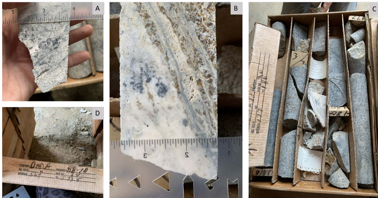
Figure 50: A) 1 ½ Core sample from DMA 88-10. B) Close up of core sample with sulfides inside matrix of carbonates. C) Image of entire core box. D) Image of lid label.
