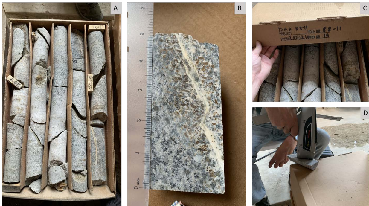
Figure 52: A) Core box for DMA 88-11, box 19. B) Image of Veinlet with weathering. C) Box lid for DMA 88-11. D) Collecting XRF data from core sample.
