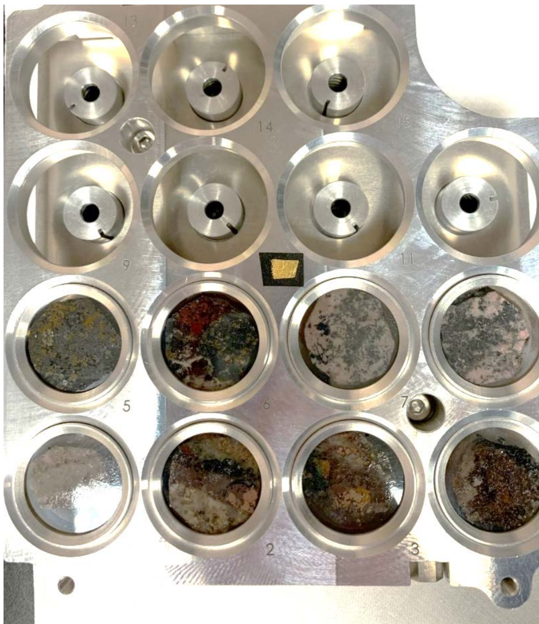
Figure 16: Loaded SEM tray with plugs that have carbon coating.
