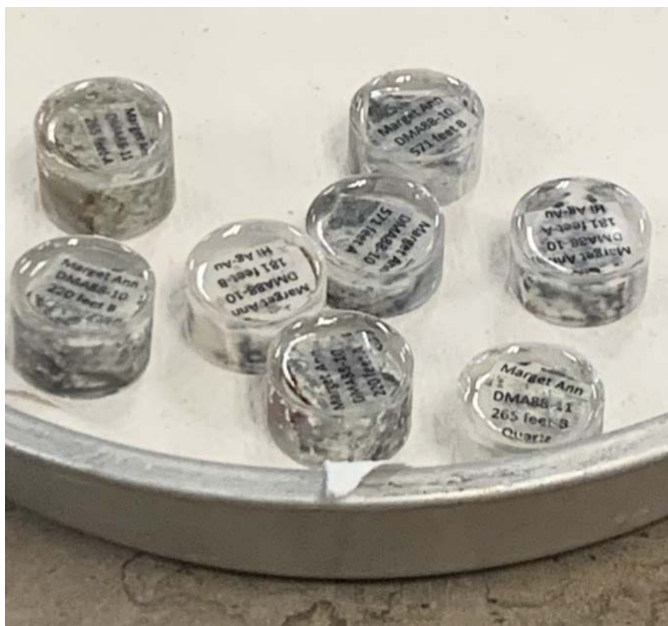
Figure 12. Example of completed resin plugs.
