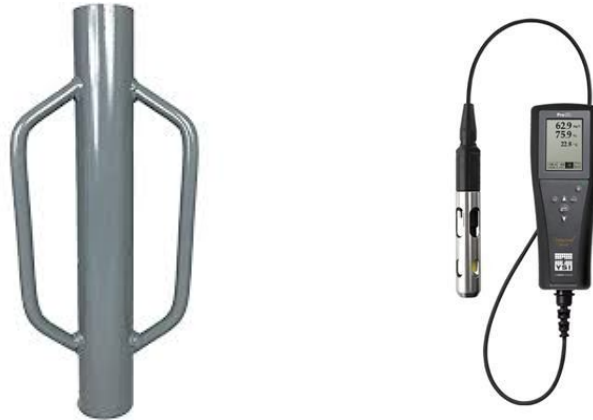
Figure 5: Hand held post pounder used to install shallow wells at sites 4-1 (right) and YSI Pro30 conductivity meter used to determine specific conductivity, conductivity, and temperature.
