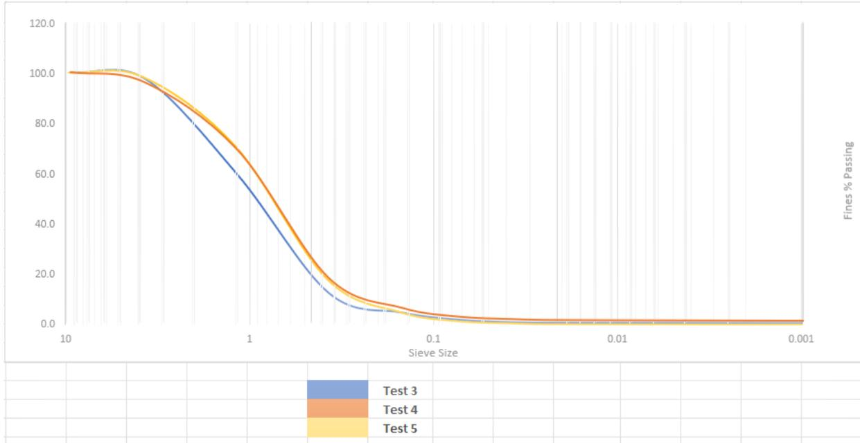
Figure 9: Sieve analysis fines percent passing, three tests are overlapped to show the similarities in passing sizes.
