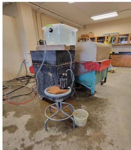
Figure 6: 1 shows the cylinders for bulk density testing, 2 shows the permeability testing
