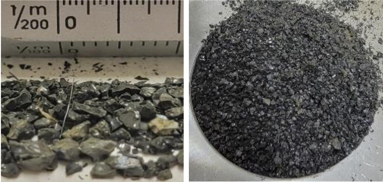
Figure 3: 1, Shows closeup of slag particles next to a 1/200 m (5.00 mm) ruler. Sizes range from below measurement to a larger 1 mm of amorphous material. 2, shows slag particles in a cylinder immediately after shear test.
