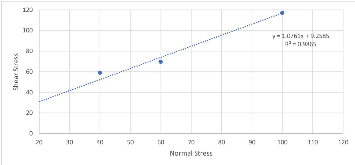
Figure 10: Max shear graph trendline showing the friction angle at 47.8° and the cohesion is 9.25 kPa
