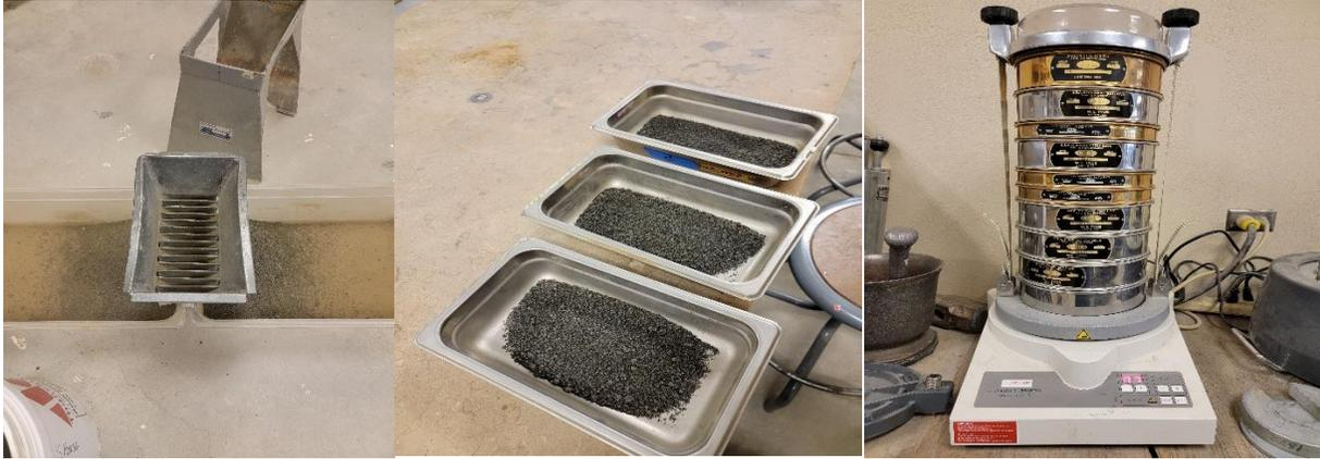
Figure 7: Preparing water-cooled slag for sieve testing. Sieves used per ASTM guidelines.
