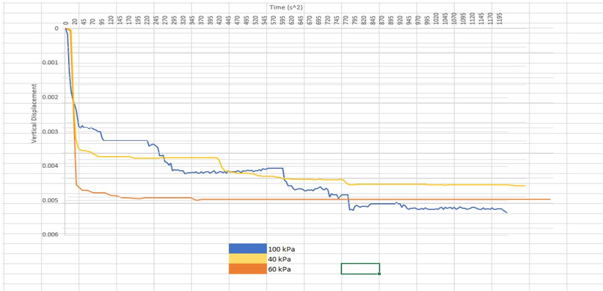
Figure 11: Consolidation phase before the shear test, this figure is at 100 kPa, tests were done using 40 kPa, 60 kPa, and 100 kPa. This figure was chosen as all tests were relatively similar in consolidation when overlapping the data onto one graph.
