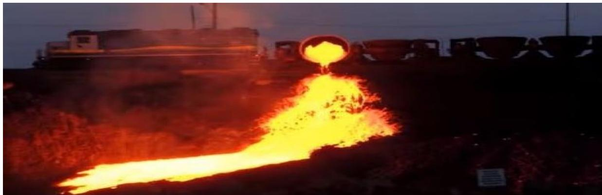
*Figure 1: Molten slag being dumped by railway*
