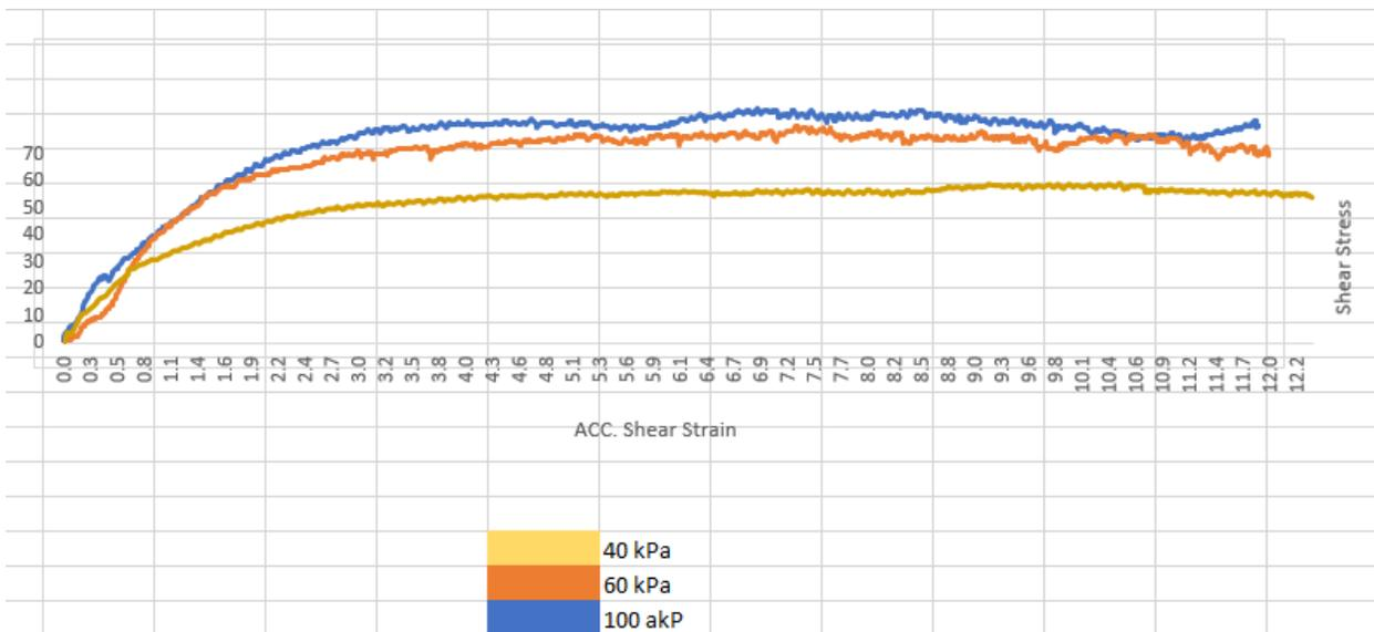
Figure 12: Shear stress vs shear strain testing, all tests were relatively similar in where the stress and strain occurred at the 40 kPa, 60 kPa, and 100 kPa marks.
