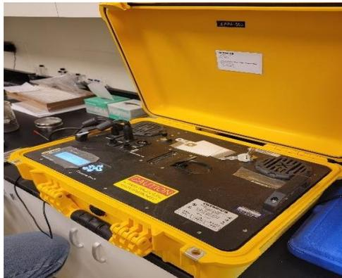
Figure 4: Using the Olympus TERRA Portable XRD analyzer to get a more precise determination of minerals in the sample. The sample used was approximately 15 mg.
