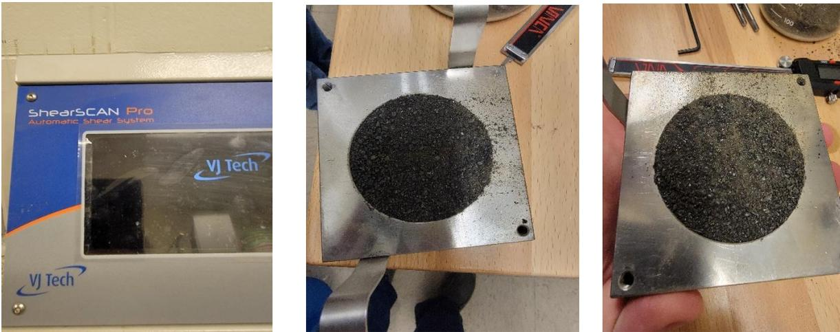
Figure 8: Shows shearSCAN Pro, and two samples that a shear test was conducted on
