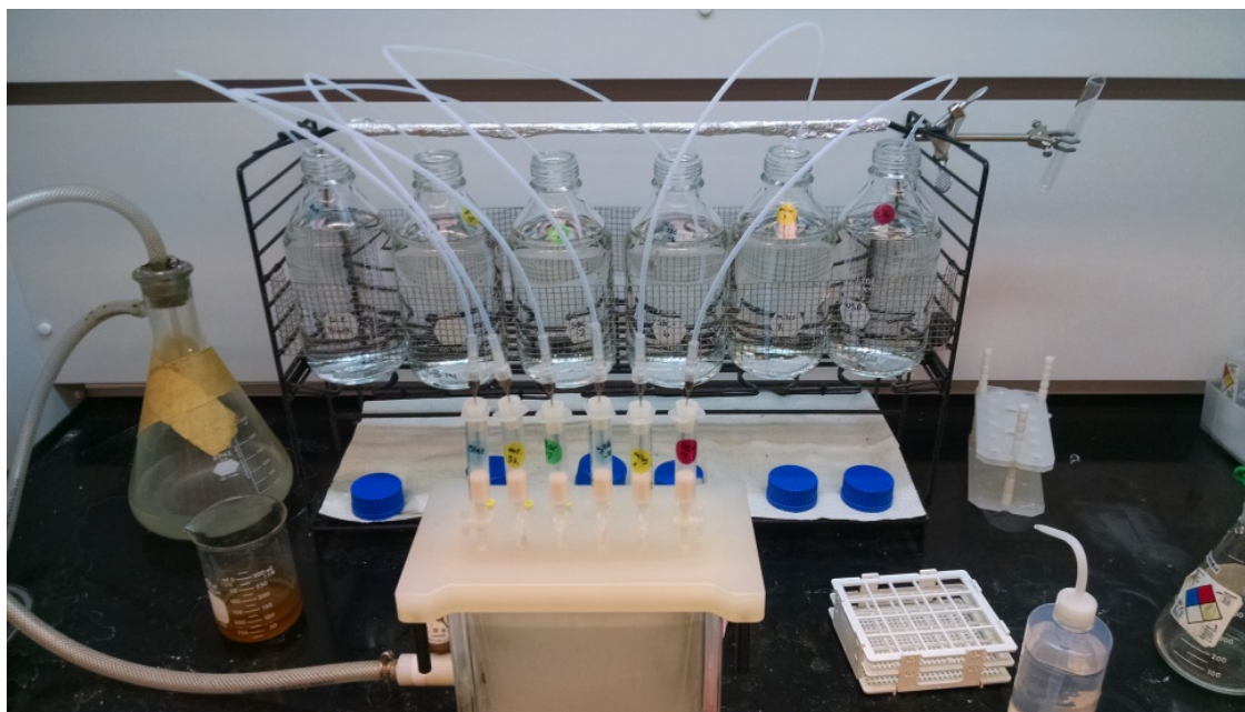
Figure 8. The set-up for the SPE extraction cartridges with leur-lock fittings and tubes for transfer of water through the cartridges.
