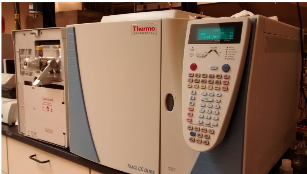
Figure 9. Thermo scientific Trace GC Ultra gas chromatograph and Thermo ion trap mass spectrometer
