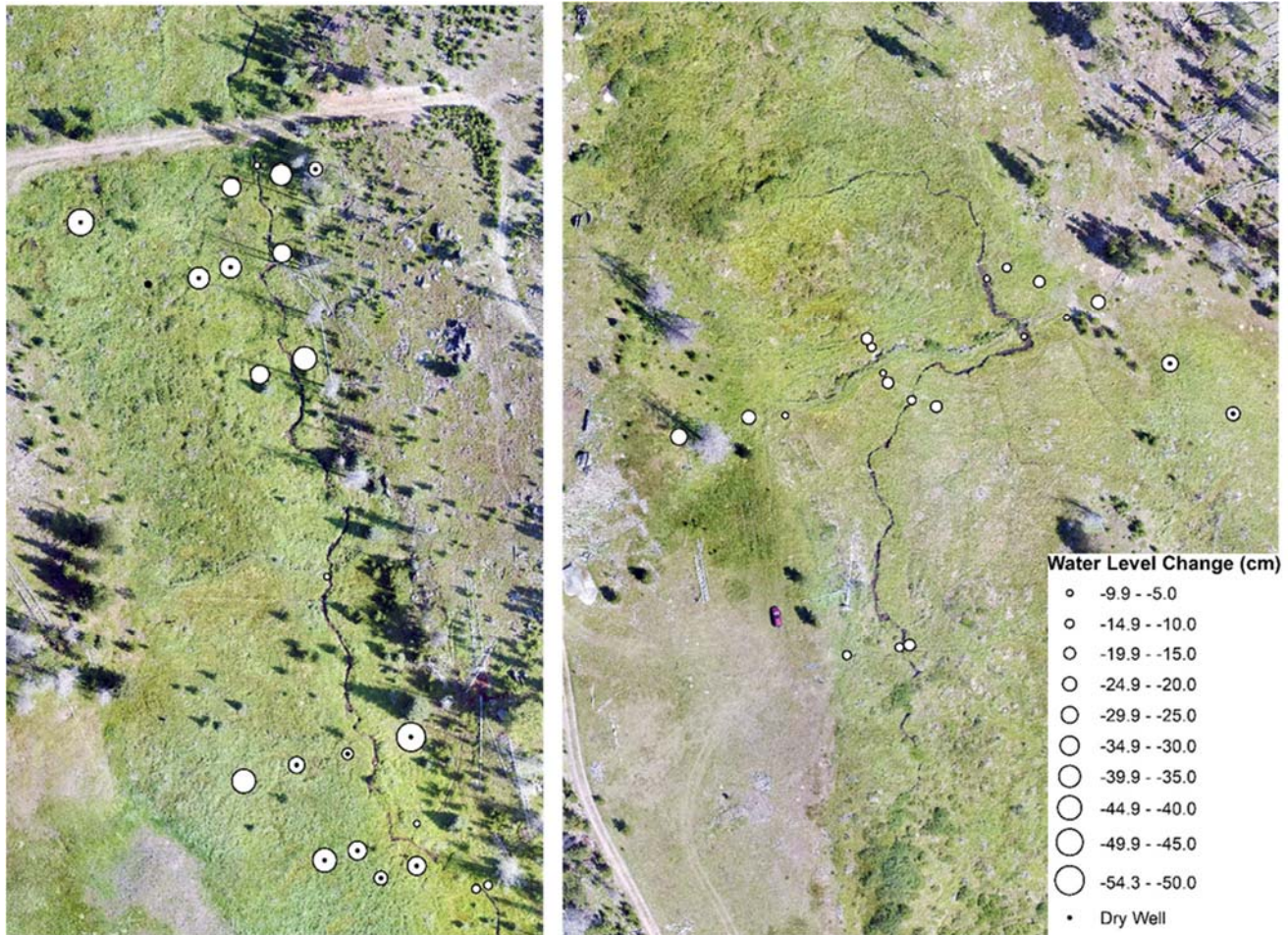
Figure 6: Blacktail Creek June-August 2019 groundwater level change on control reach (left) and treatment reach (right)
