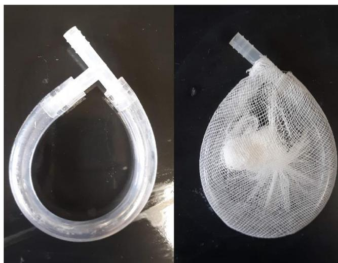
**Figure 5. Permeable Barriers used to Separate Electrode Compartments from Soil.**
