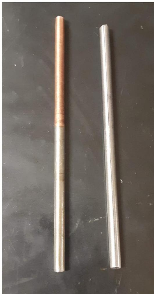
**Figure 11. Copper Plating on Positive EDTA Electrode after polishing.**
