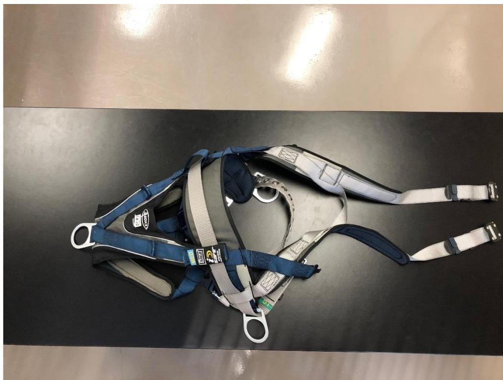
**Figure 2. DBI Sala ExoFit full body harness exhibited before repetition**
