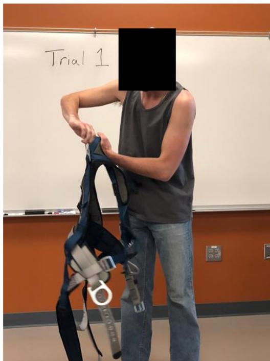
**Figure 5. Participant grabbing the D-ring of harness to begin shake out portion**
