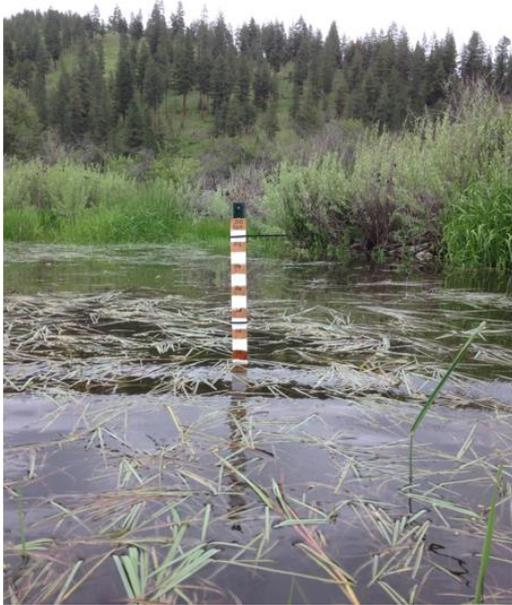
**Figure 9: Staff gauge installed in a tailings pond at the GTS**
