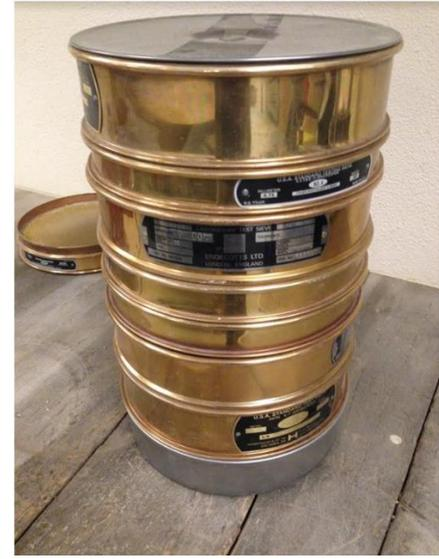
**Figure 12: Soil sieves setup in accordance with ASTM D6913.**
