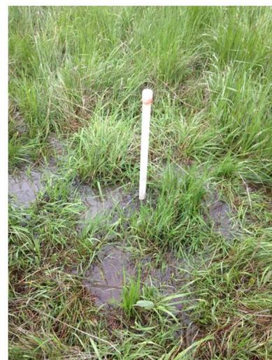
**Figure 8: Monitoring well installed at GTS**
