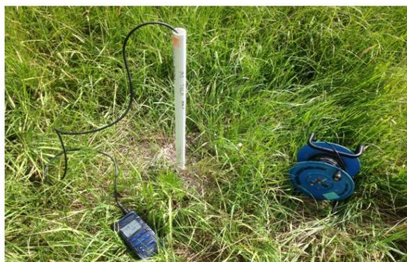
**Figure 10: Multi 340i probe measuring temperature and specific conductivity in a monitoring well**
