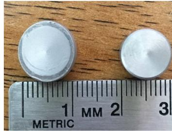
**Figure 13: Comparison of a 0° specimen tested at  $2.5 \times 10^3$  /s strain rate (left) and an untested specimen (right)**
