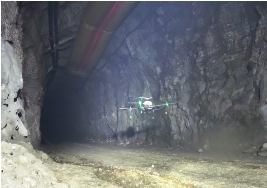
Figure 17. Near Earth Autonomy's M2 platform autonomously navigating the 995-480 drift.
