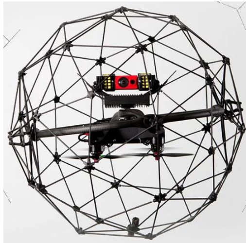
Figure 19: Flyability’s Elios platform. The UAV and camera are mounted on a detachable gimbal so the carbon fiber cage can freely rotate around it. The propellers are located on the bottom of the UAV so that the camera and LEDs (shown in red) can be located on the top.
