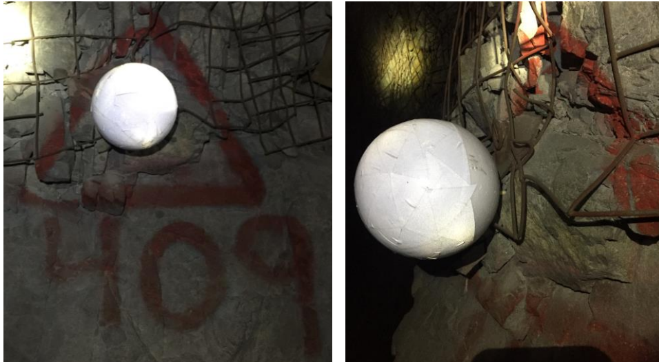
Figure 5. Several 6-inch diameter reflective foam balls were placed in survey collars along the flight path to be used as ground control points (GCPs). GCPs were placed in mine survey monuments using wooden dowels.
