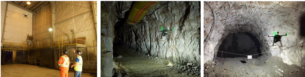
Figure 4. Examples of different flight types including the (left) surface wash bay, (center) underground drift flight, and (right) underground stope flight.
