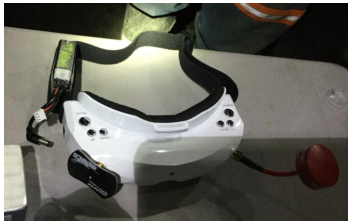
Figure 14. First-person view (FPV) goggles used by the pilot to view a live video feed from the UAV during flight.
