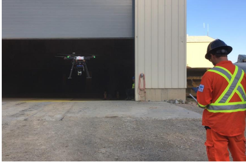
Figure 8. The Hovermap Standard payload entering the surface wash bay as a stope simulation.
