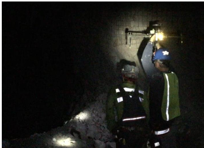
Figure 18. The M2 platform was held near the entrance to the 945 stope to measure the stope with the VLP-16 LiDAR scanner without completing a flight.
