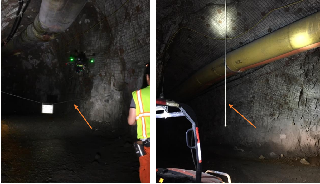
Figure 9. The Hovermap Mining payload obstacle detection system was able to identify a rope barricade across the drift ( left ) and a rope hanging from the roof ( right ).
