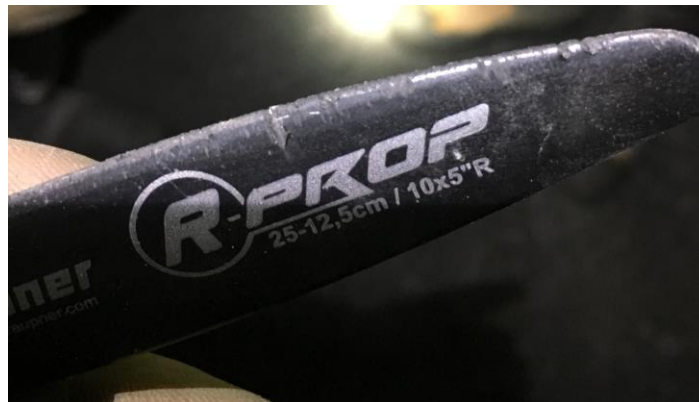
Figure 13. Wear to the Ranger propellers from dust in the air during flight.
