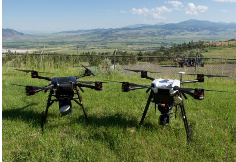
Figure 6. Emesent’s Hovermap Mining payload ( left ) and Standard payload ( right ).
