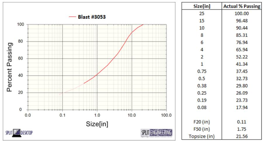
Figure 10: Fragmentation Size Distribution for Blast #3053
