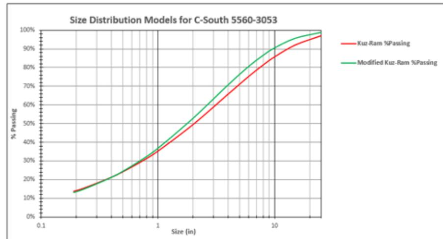
Figure 9: Kuz-Ram and Modified Kuz-Ram models in MS Excel 2016
