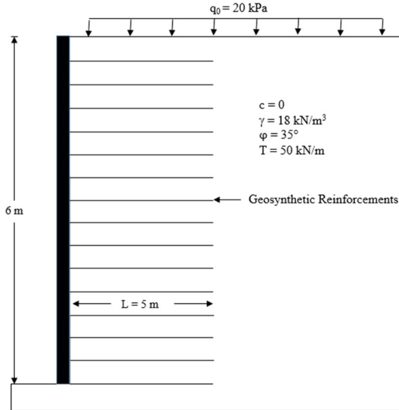
**Figure 1. Schematic of Geotextile Reinforced Soil Wall**
