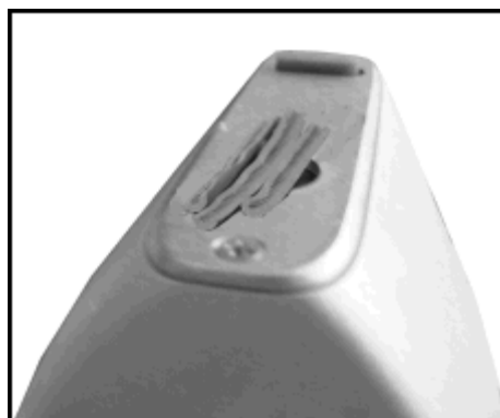
Figure 17. PVC Wire Insulation With Conductor Removed
