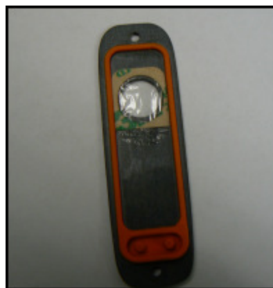
Figure 6. Measurement Window Replaced
