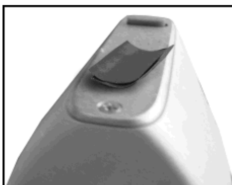
Figure 19. Correct Way to Measure Heat Shrink Tubing
