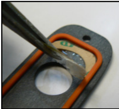
Figure 2. Removing the Old Window
