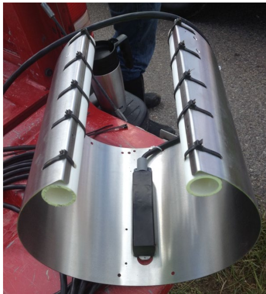
Figure 1. Spring ring ready for installation.
