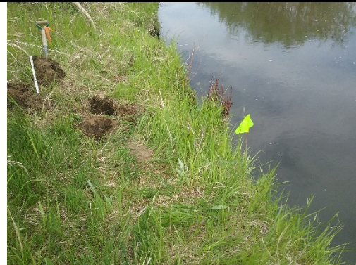
Plot 10. Green flag indicates end of delineation at stream edge. Excavation did not indicate saturation within 16 inches of surface.
