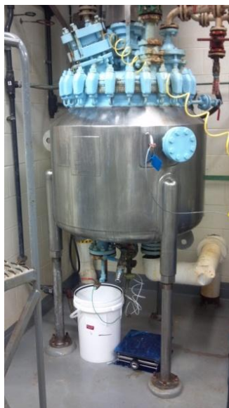
Figure 4: Bucket staged below reactor to capture separated layers.
