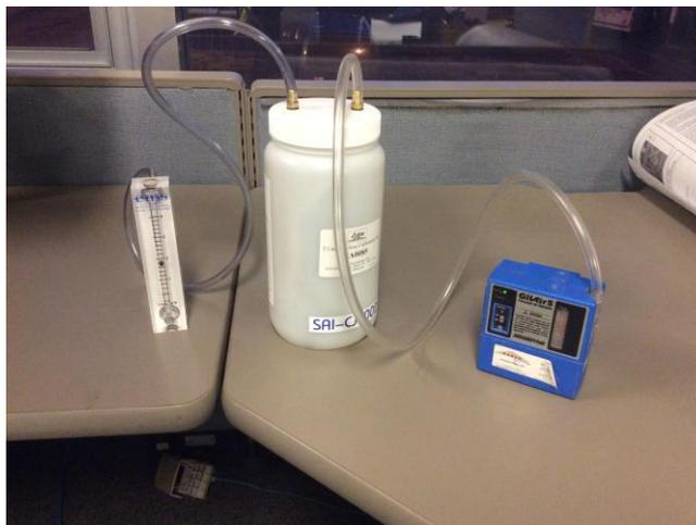
**Figure 1: Sampling pump calibration**
