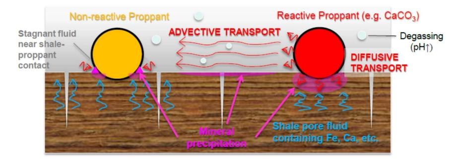
Reduce fracture deformation and proppant embedment via mineral precipitation.
