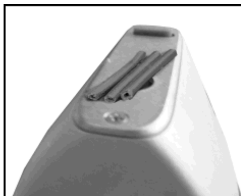
Figure 16. Wire Insulation Cut Into Strands
