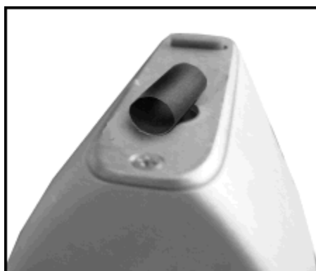
Figure 18. Incorrect Way to Measure Heat Shrink Tubing
