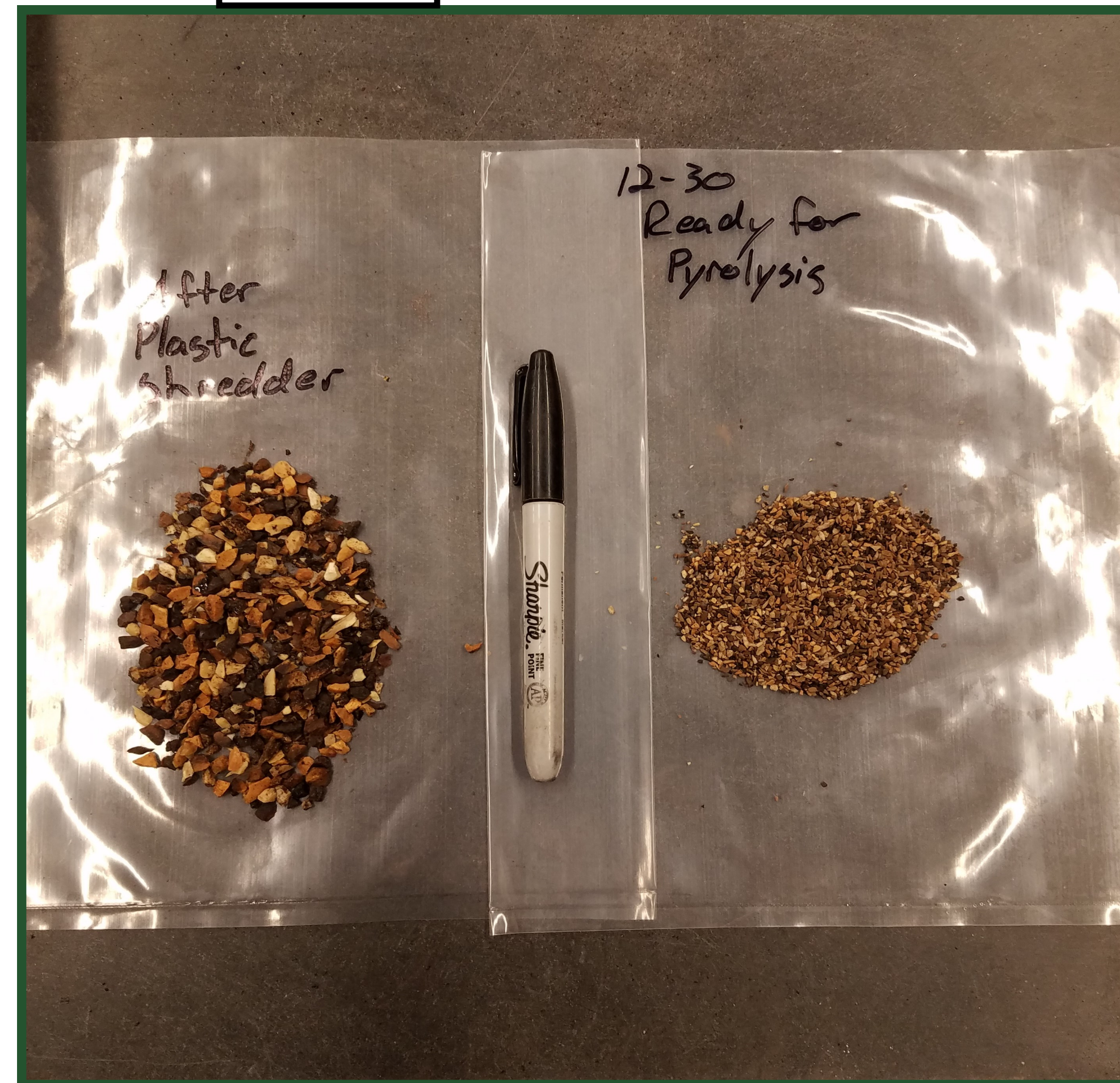
Sized bone char before pyrolysis
