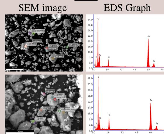
EDS graphs verify that silica was coated on the  $\text{Fe}_3\text{O}_4$  NPs.
