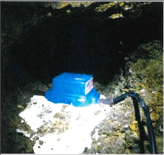
Figure 17. Geophone installed in 6 inch hole.
