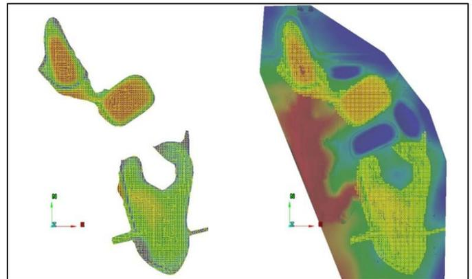
**Figure 1.** GPS Survey (left) and UAS Survey (right) with common 6 meter grids.
