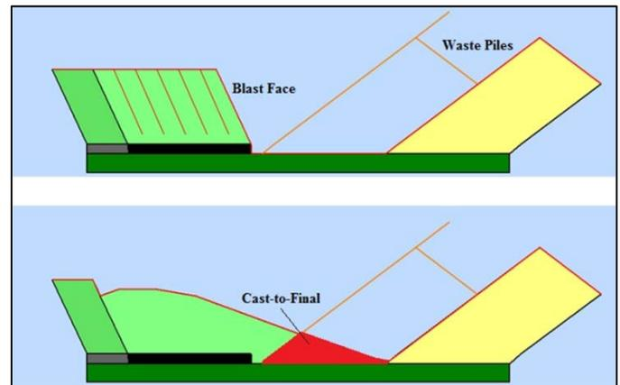
**Figure 1.** A cast profile shows a cast blast before and after the overburden was blasted.
