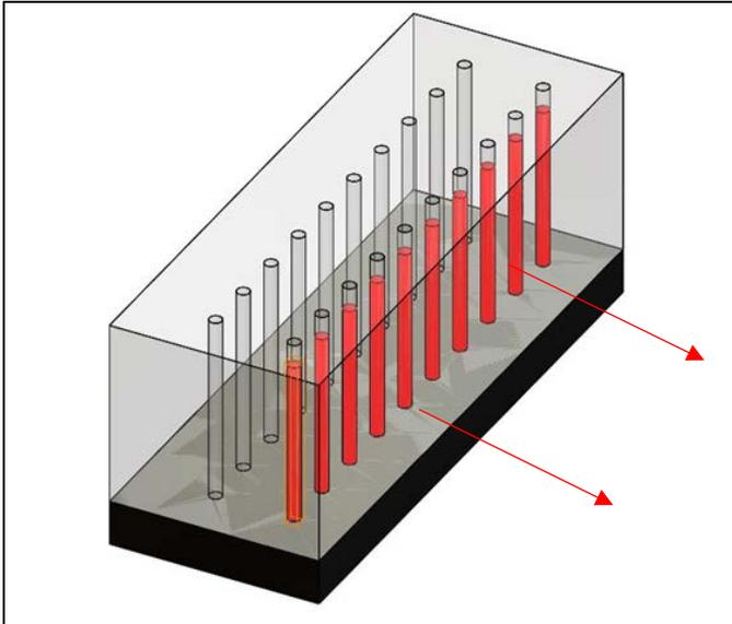
**Figure 2.** A 3-dimensional concept drawing of how a traditional cast blast is drilled and the relation of the drill holes to the blast face. The arrows represent the blasted material movement direction.
