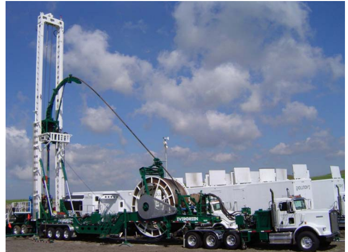
Figure 7. A typical coil tube drill rig used in the petroleum industry. This type of drill rig is loaded on a trailer and is able to be moved relatively easy (Foremost, 2016).
