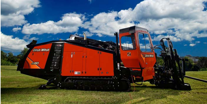
Figure 8. This type of drill rig is used for utility line installation (Ditch Witch, 2015).
