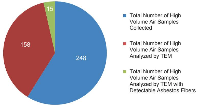
Two hundred forty-eight high-volume samples were collected (excluding field sample blanks) and analyzed by phase contrast microscopy. Of these, 158 were further analyzed by transmission electron microscopy (TEM). Fifteen of the TEM air samples revealed detectable asbestos fibers.
