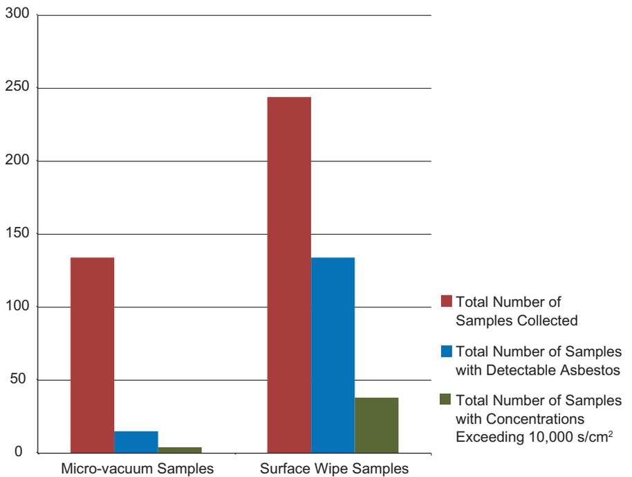
One hundred thirty-four micro-vacuum surface samples and 244 surface wipe samples were collected. Of these, 23 and 134 micro-vacuum and surface wipe samples, respectively, revealed detectable asbestos fibers. Four micro-vacuum and 38 surface wipe samples revealed asbestos concentrations exceeding the 10,000 s/cm<sup>2</sup> concentration adopted as the background surface concentration for our study.
