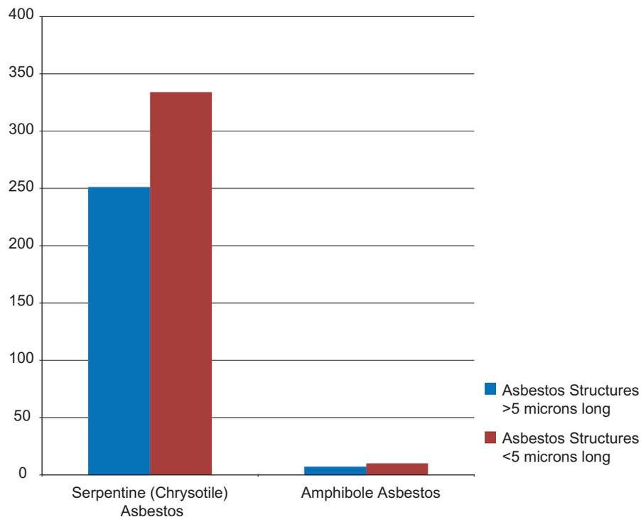
In terms of individual asbestos structures identified in surface wipe samples, 585 structures were chrysotile while 17 were identified as Libby amphibole or actinolite/tremolite. Asbestos structures less than 5  $\mu\text{m}$  are distinguished from asbestos structures greater than 5  $\mu\text{m}$  for both families.
