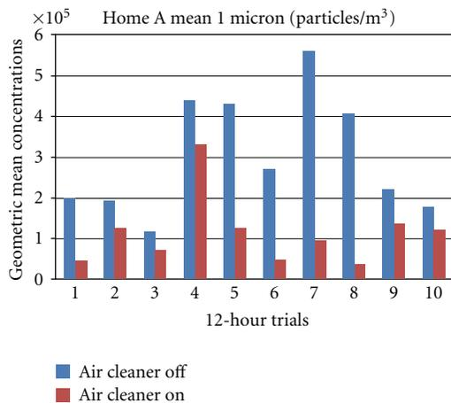
FIGURE 2: Geometric mean particle count concentrations ( $\text{particle}/\text{m}^3$ ) observed with the portable air purifier off and on at the one  $\mu\text{m}$  cutpoint for each 12-hour trial conducted in home A. Concentrations recorded with the air purifier on were consistently lower than concentrations recorded with the air purifier off. Similar observations were made in terms of particle concentration reductions with the air cleaner on at the other cutpoints.
