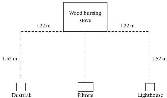
FIGURE 1: Configuration of the wood burning stove, Filtrete air purifier, DustTrak aerosol monitor, and Lighthouse particle counter in each home. An additional DustTrak was placed in a secondary location (bedroom) 5.84 meters from the wood stove in Home B.
