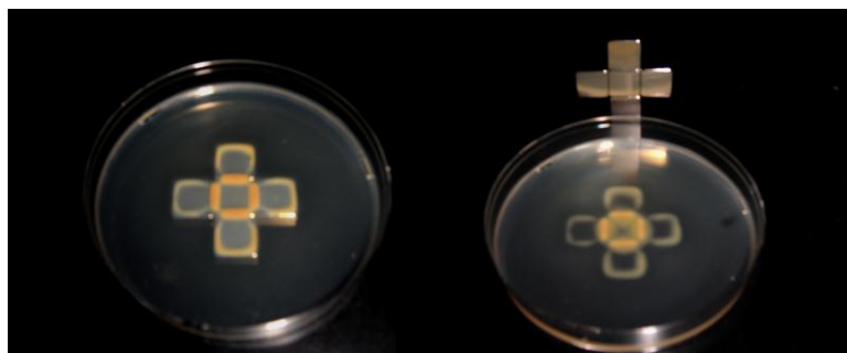
Fig.2 Photograph showing the assembly of complex shapes of Fe doped in HA using the citrate capping synthesis technique.
