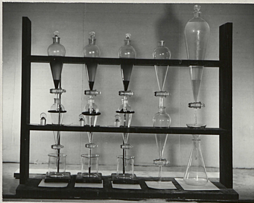
Fig. 2. Apparatus Used in the Separation of Heavy Minerals from Light Minerals.
