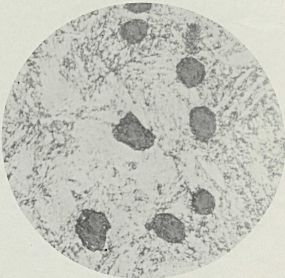
Small, nodular rosettes of pearlite in a matrix of martensite that was slightly tempered during grinding and polishing.
