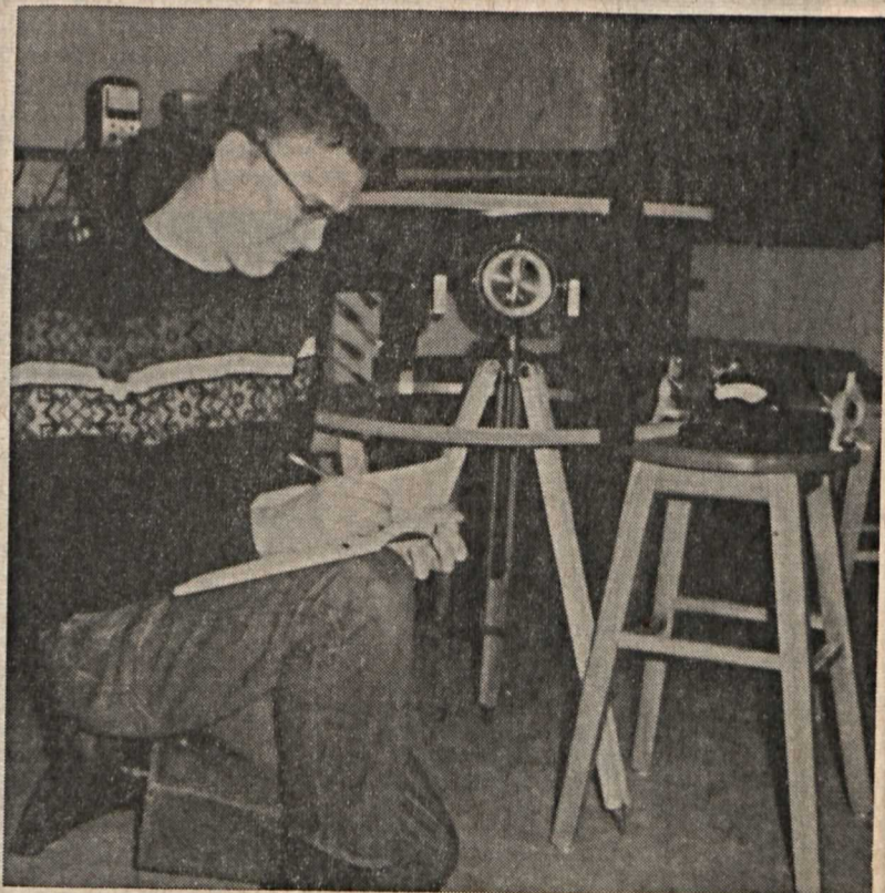
Bob Heaphy, a senior in Geophysical Engineering, makes a correction on a magnetometer with a helmholtz coil.
