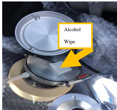
Figure 5. Alcohol wipes were used to clean and disinfect the Andersen sampler between collections.
