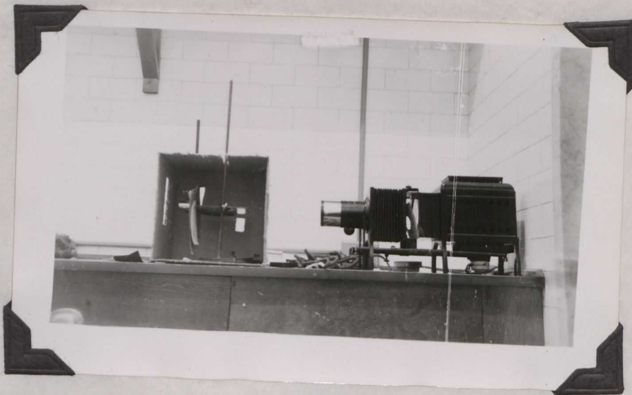
Projector, Ocular Lens, Specimen Holder
