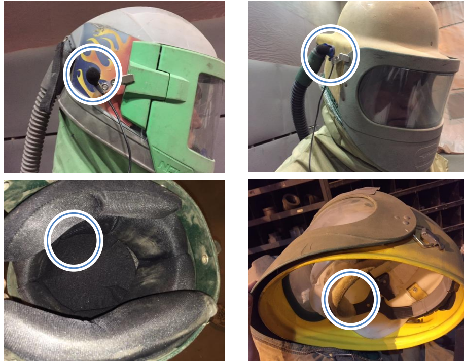
Figure 2 - Nova 2000 Blast Helmet (left) and Bullard GenVX Blast Helmet (right) with dosimeter microphones installed.
